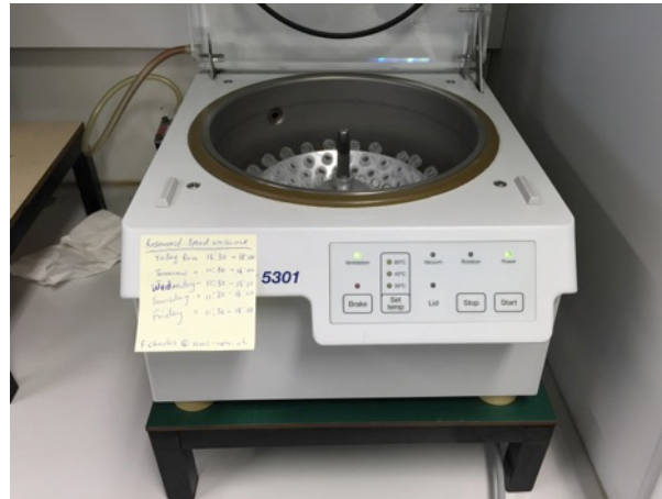
Figure 4. Evaporation of ammonium by centrifuge and vacuum at 60 °C
